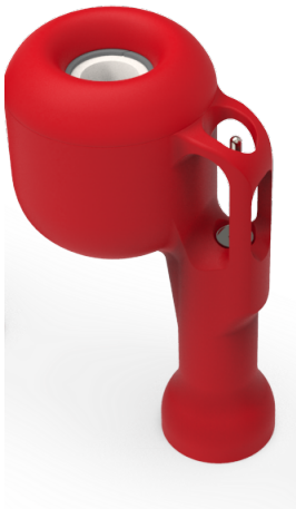
Fig. 1 The 2000dbar RBR combined conductivity-temperature (CT) cell. The temperature sting is vertically aligned with the conductivity cell, minimizing errors caused by CT separation.
